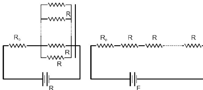
The batteries in both circuits are identical and net power dissipated in the  $n$  resistors in both circuit is same. The ratio  $R_0/R$  is :
